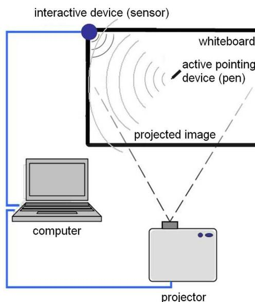
Picture 1. Working principle of an interactive whiteboard
